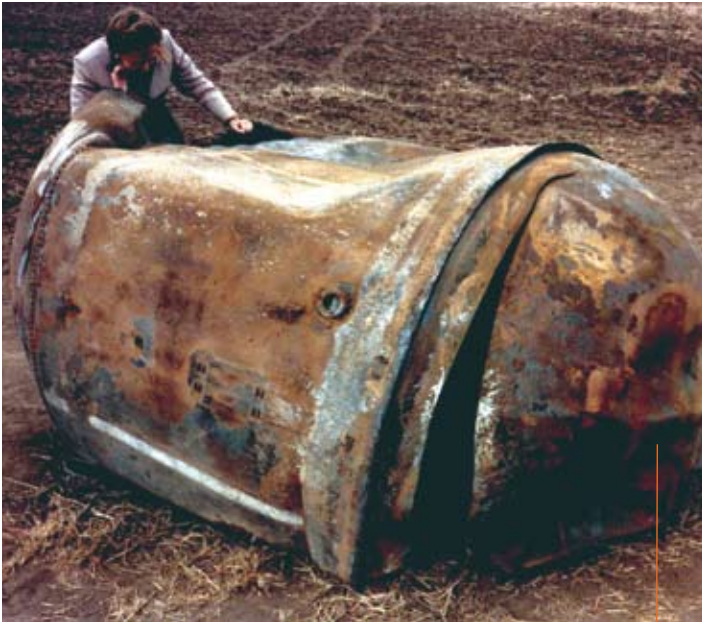
This is the main propellant tank of the second stage of a Delta 2 launch vehicle, which fell from space and landed near Georgetown, TX, on 22 January 1997.
