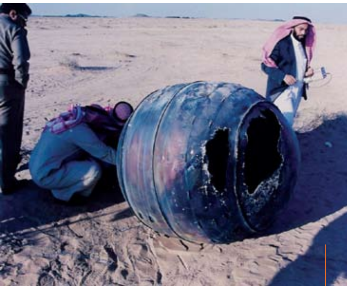
On 21 January 2001 a Delta 2 third stage reentered the atmosphere over the Middle East. The titanium motor casing, weighing about 70 kg, landed in Saudi Arabia about 240 km from the capital of Riyadh.
